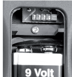
Figure 7: DIP Switch in Remote Handset Battery Compartment
